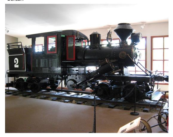
Restored Climax logging locomotive on display at the BC Forest Museum in Duncan. This unit operated in the Lake Cowichan area from 1911 to 1924 and then was abandoned in the bush. It was taken out in 1970 and "reassembled" with odd truck parts. In 1975, it was refurbished and made operational by BC Forest Products who then donated it to the BC provincial museum. Photo by A.C.
